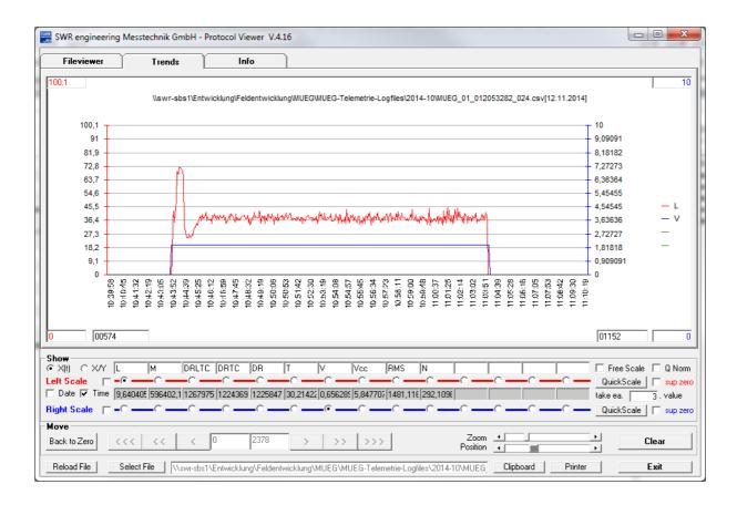
After starting the loading the controller adjusts the flowrate by getting the feedback from the MaxxFlow sensor. The flowrate overshoots and undershoots only one time until loading is performing with constant (controlled) flow rate. After the integator has reached the desired preset-value the conveying stops.
