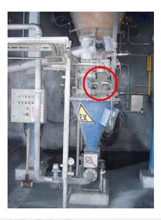
Simple measurement and regulation of lime addition during the flue gas cleaning. Regulation of the rotation speed of a screw feeder through the amount of material measured by the SolidFlow depending on the measurement of the filtered gas.
