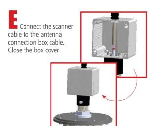
The Head Mounting part is supplied with the extension cable wired.
